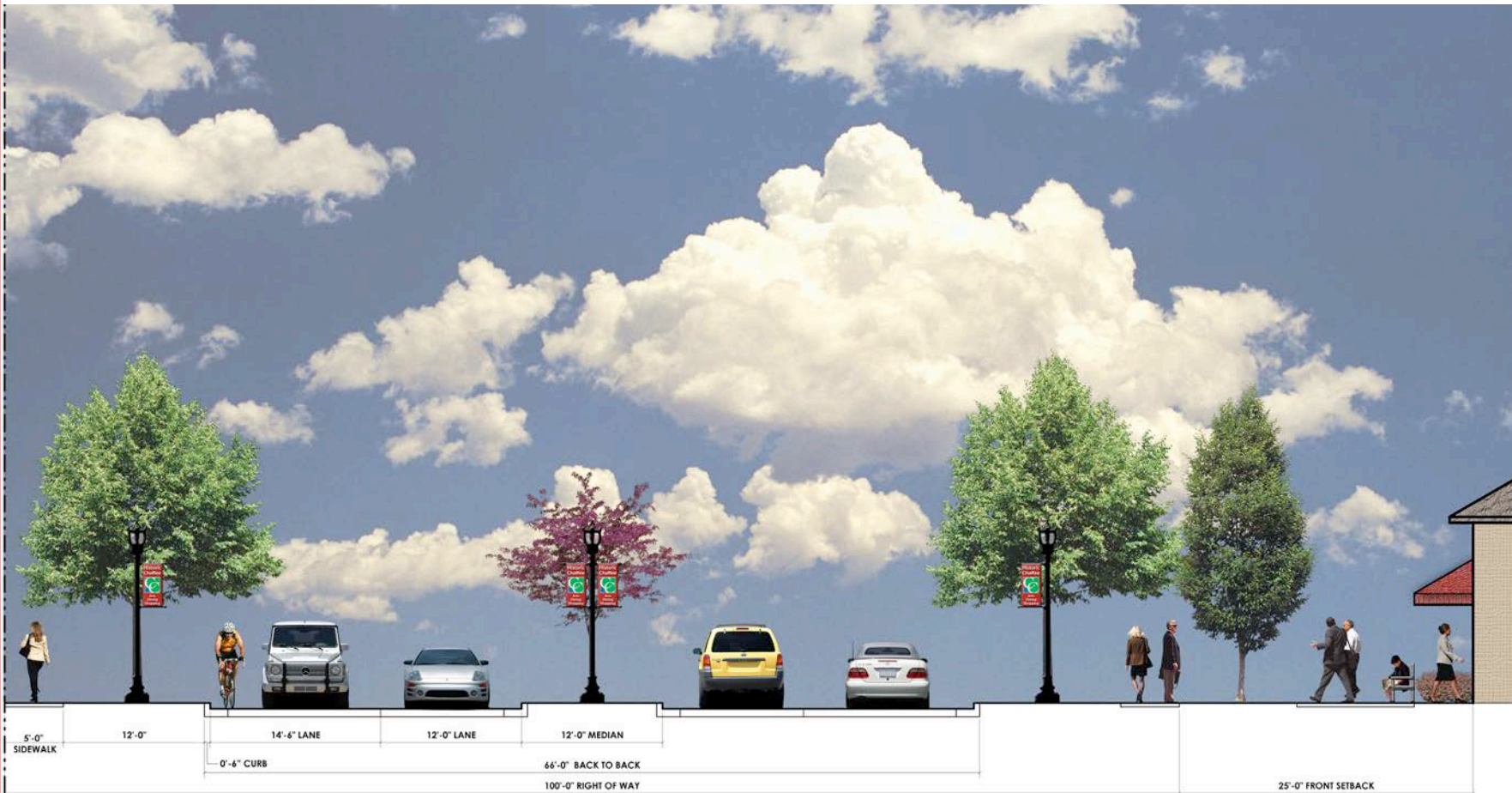
EXAMPLE: MAJOR ARTERIAL WITH CONTROLLED CENTER TURN LANE (derived from Fort Smith's Major Arterial with continuous center turn lane)
